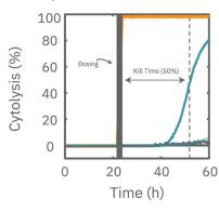
(Left) After application of doxorubicin (Dox.), the impedance measurements revealed the dynamic response of the A549 cells compared to (middle) the single time point values shown at the dotted line. (Right) Using on-plate controls for cell growth (No Treatment Control) and cell death (Tergazyme), the percent cytolysis was tracked in real time throughout the time course of the response.
